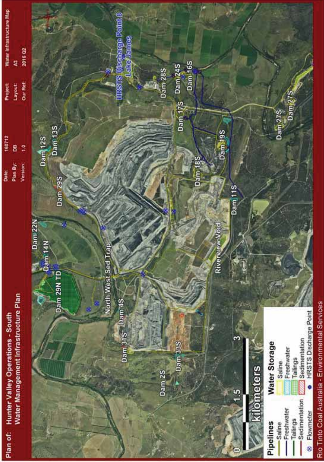
Figure 27: South Pit water management infrastructure
